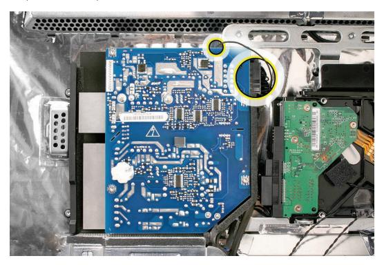
4. This shows a close up of the two-pin ground cable connector on the underside of the power supply.
